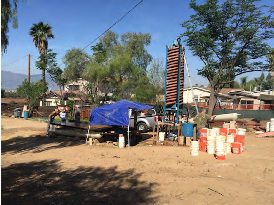
Bulk testing activities of Poker Game Mine ore, March 2016. Ore was crushed and screened to 30 mesh, mixed into a slurry, pumped into a spiral separator and concentrates ran over a shaker table. Approximately 4.5 tons of ore was processed.
