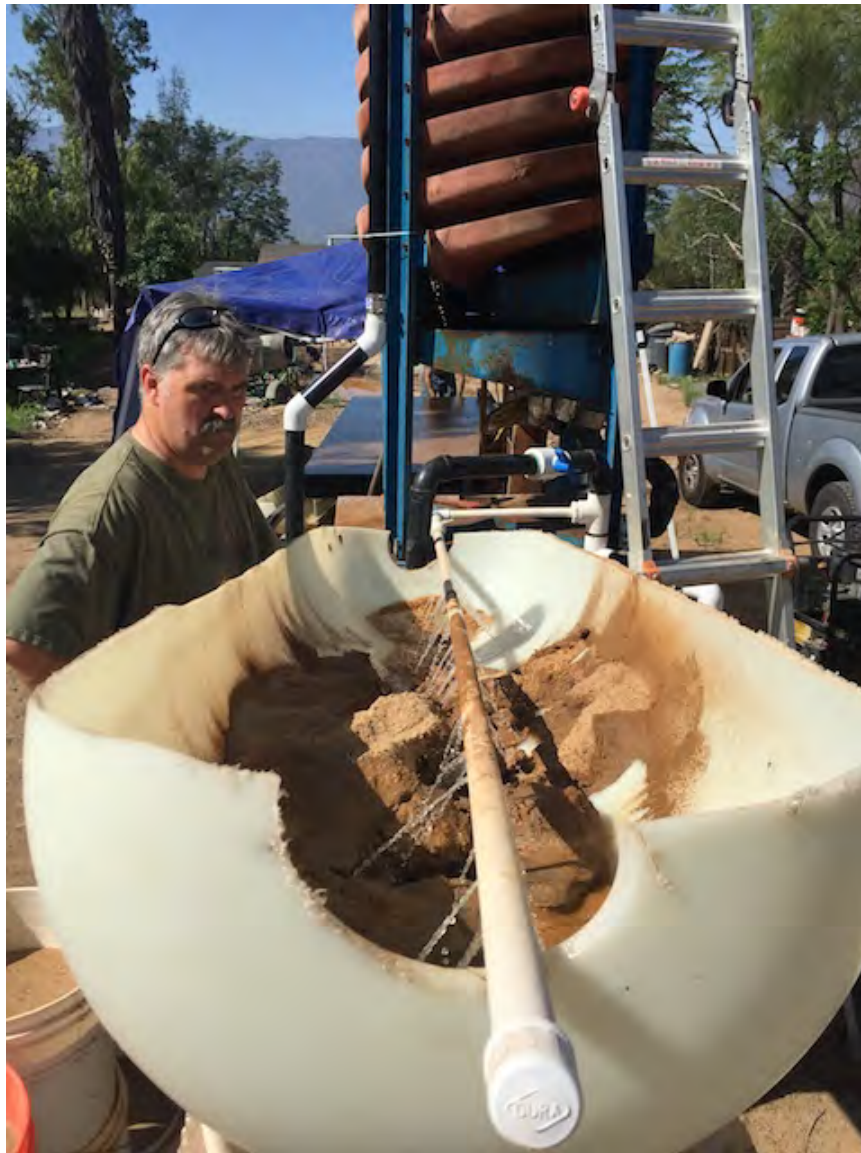
Crushed ore mixed into a slurry and pumped to a spiral separator.
