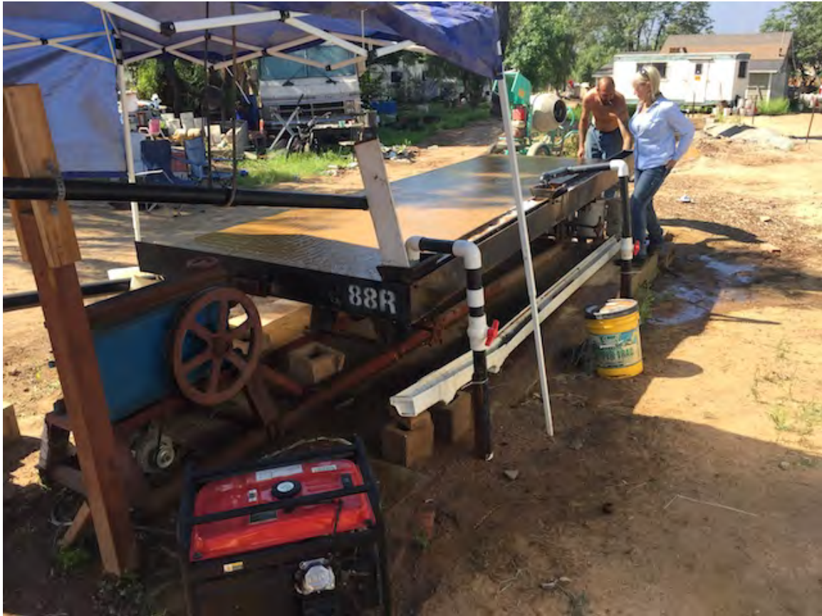
Concentrates from spiral separator are run across a 16-foot shaker table.
