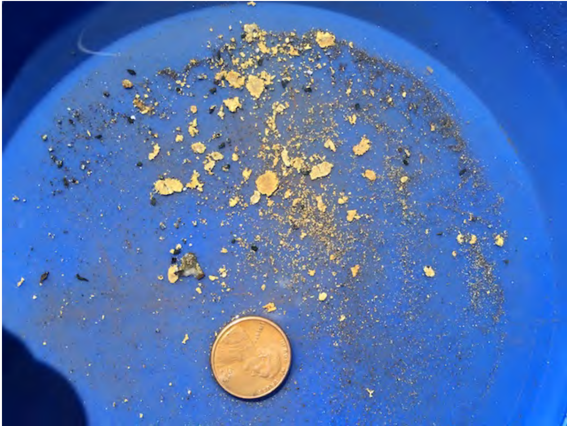
Coarse-grained gold caught in spiral separator trap. Notice the flattened texture from the roller mill crushing process - like pennies on a railroad track. This indicates the Poker Game Mine contains coarse-grained gold, which requires an addition to a production-grade processing facility.
