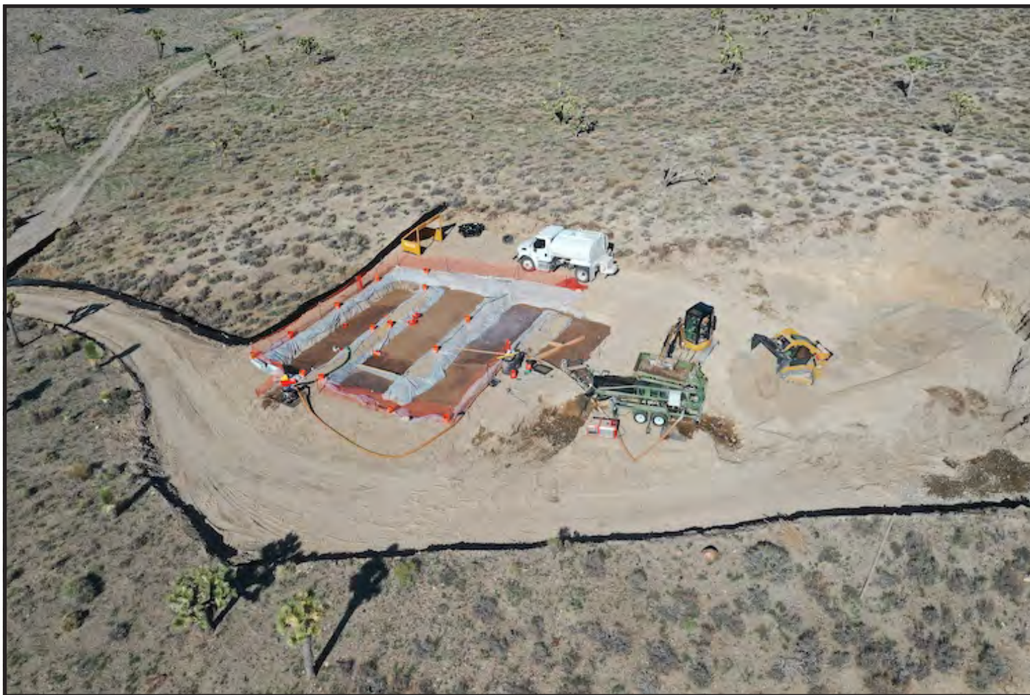
Photo 7. Drone overview of the Phase 1 Exploration and Bulk Testing processing area. The processing area occupied an area of about 150 feet x 100 feet or roughly 15,000 square-feet. The processing area consisted of a stockpile area, a level pad for a trommel, and a series of four plastic-lined ponds, three that are approximately 20 feet x 40 feet x 8 feet deep and used as clarifying ponds and one that was used as a tailings pond that was approximately 20 feet x 25 feet x 8 feet deep. The ponds were lined with plastic sheeting and linked in series so that the water flowed from one and to the other, and so on and is clarified and recirculated.
