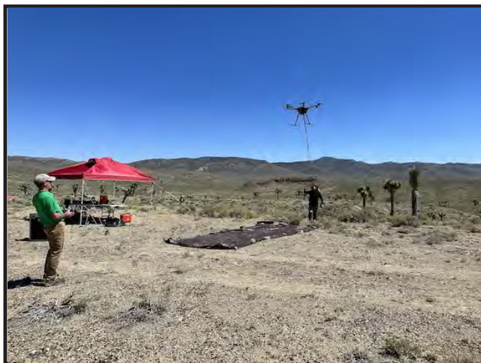
Photo 5 A. Advant used a grid pattern to acquire the data from the DJI Matrice 600 Pro UAV, a hexacopter with excellent flight performance and good load capacity. The UAV uses a Flight Controller A3 system for navigation and a SF11 Laser Altimeter to maintain the proper altitude over the targeted area.
